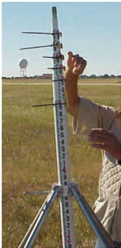
Figure 6. WRK Drift Tower
